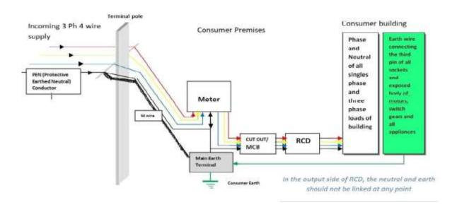
• The protective earth wire should not be linked with the neutral at any point of wiring installation after the RCD location. If protective earth wire and neural are linked after RCD location, the tripping of RCD would be affected defeating the purpose of RCD. Looping of earth wire at three pin plug point with neutral should not be done.
