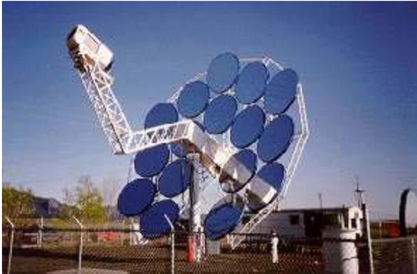
The solar dish generates electricity by focusing the sun's rays onto a receiver, which transmits the heat energy to an engine. The engine is a sealed system filled with hydrogen, and as the gas heats and cools, its pressure rises and falls.
